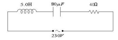
(a) Determine the source frequency, which drives the circuit in resonance.
